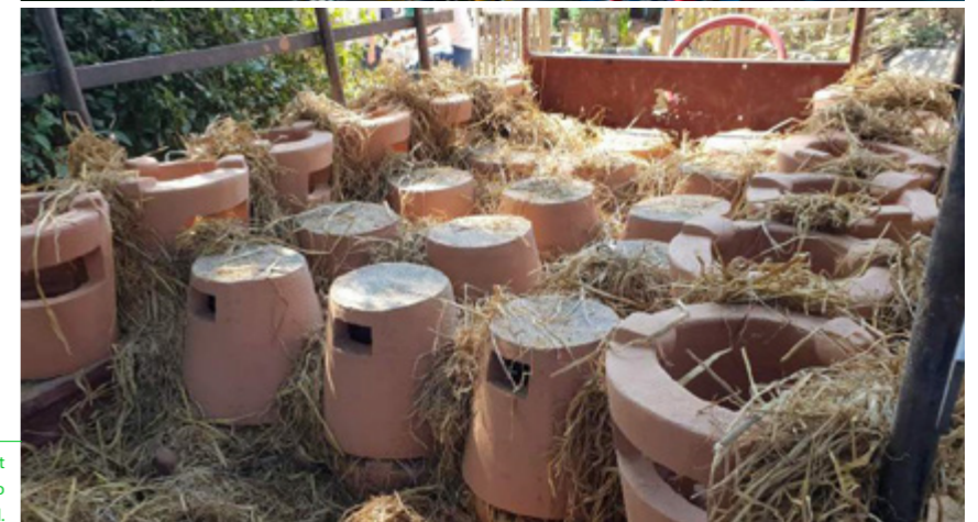
By distributing cooking utensils(cookstoves) with low heat loss to ordinary households in Myanmar, it is possible to reduce the amount of wood consumed as fuel.
